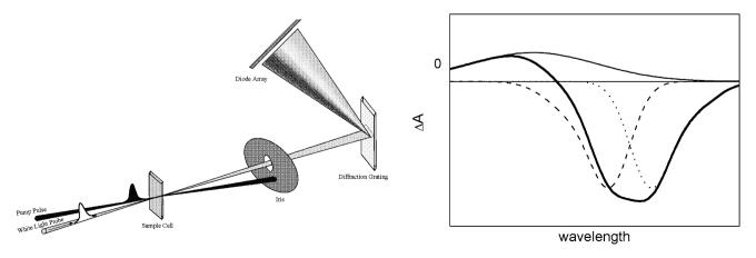
Fig. 1 Left panel: Schematic depiction of the transient absorption spectroscopy principle. Right panel: Contributions to a  $\Delta A$  spectrum: ground-state bleach (dashed line), stimulated emission (dotted line), excited-state absorption (solid line), sum of these contributions (gray line)
