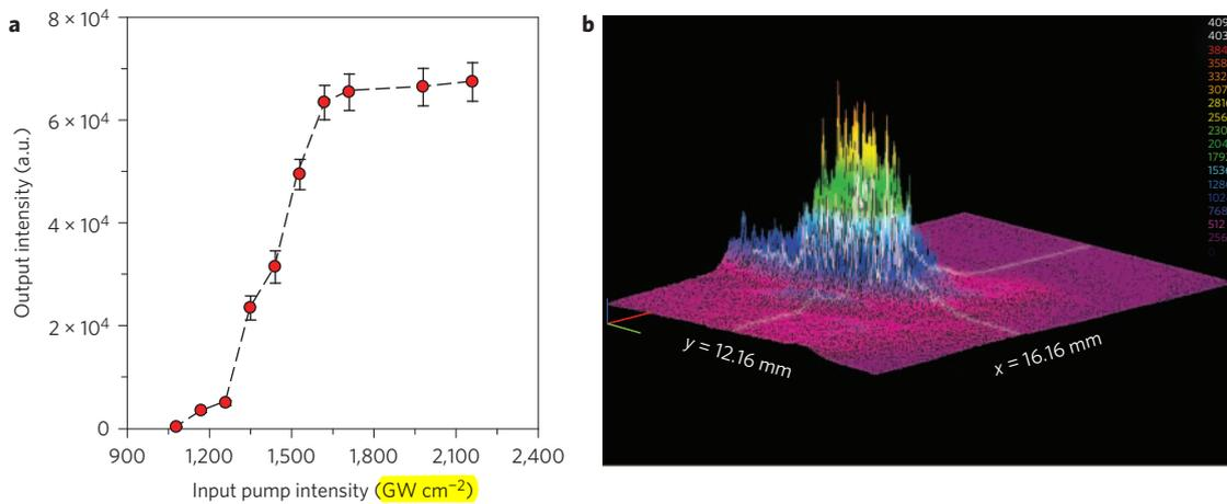
**Figure 4 | Output/input power characteristics and far-field distributions of 5PP stimulated emission.** **a**, Output/input power characteristics for 5PP stimulated emission from IPPS solution (0.15 M in DMSO-d<sub>6</sub>). **b**, Far-field distributions of the 5PP stimulated emission beam. Error bars indicate experimental uncertainty of ±10%.
