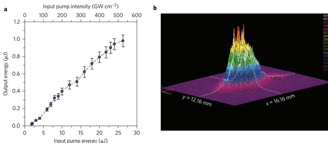
**Figure 3 | Output/input power characteristics and far-field distributions of 3PP pumped stimulated emission.** **a**, Output/input power characteristics for 3PP stimulated emission from IPPS solution (0.15 M in DMSO- $d_6$ ). **b**, Far-field distributions of the 3PP stimulated emission beam. Error bars indicate experimental uncertainty of  $\pm 10\%$ .
