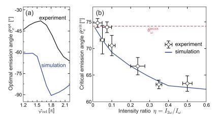
**Figure 22. (a)** Relative phase-dependent optimal emission angles for downward emission obtained from experiment (black) and simulation (blue) with 300 nm  $SiO_2$  nanospheres at  $\eta = 0.5$  (cf. black curves in Figure 21(d,g)). **(b)** Intensity ratio-dependent critical emission angles for upward emission obtained from measurement (circles) and SMM simulations (solid blue curve) with 300 nm  $SiO_2$  nanospheres. Adapted from [51] under Creative Commons Attribution 3.0 licence.
