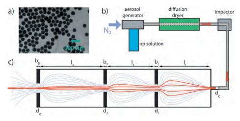
**Figure 3. (a)** TEM image of  $SiO_2$  nanospheres with a diameter of 147 nm. **(b)** Flow diagram for the generation of the nanoparticle aerosol. **(c)** Working principle of an aerodynamic nanoparticle lens. The trajectories of gas molecules are schematically indicated by the blue dashed lines. The nanoparticle trajectories are shown in red. From [62].
